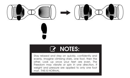
Find your center of gravity. If your weight is distributed correctly on the foot mats and your center of gravity is level, you should be able to stand on your Ultra just as if you were standing on the ground.
