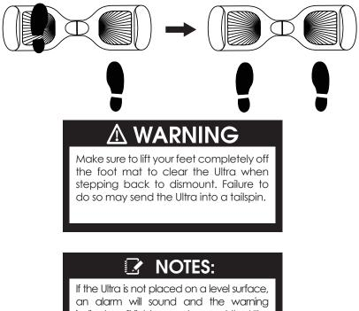
an alarm will sound and the warning indicator will light up and prevent the Ultra from moving. Place the Ultra on a level surface and try riding it again.
