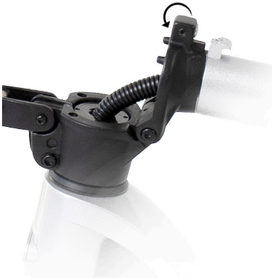
Figure 7. Remove Screw on Folding Stem
